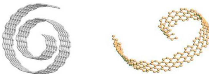
Figure 2. Folding the sheets of XY atoms to form multiple layer nanotubes.
