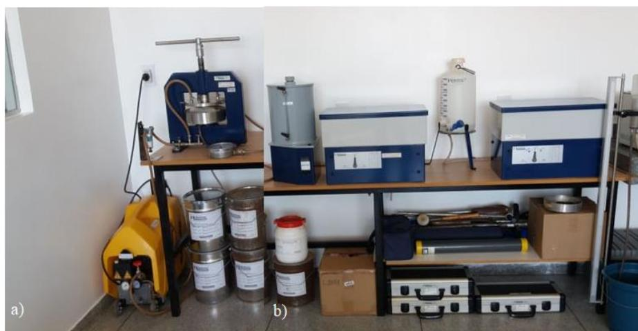
FIGURA 21 – a) extrator de membrana – Eijkelkamp (Pressure Membrane Apparatus); b) mesas de areia sintética – Eijkelkamp (Sandbox for pF -determination).
